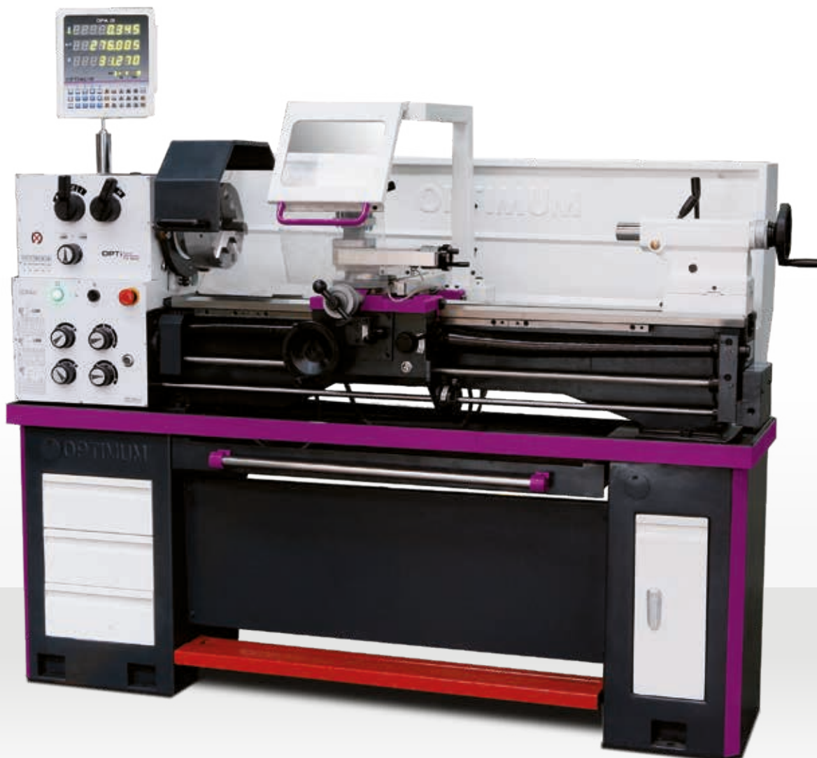
Fig.: TH 3610D - Shown with optional lathe chuck
