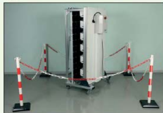
SOL-ECO2, protection by bounded safety zone
