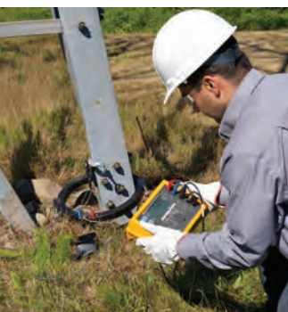
Clamp-on transformer accessory for ground loop measurements on transmission pylons.
