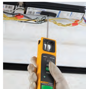
Easily determine if ballast is working.
